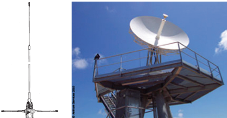
Figure 43: Left, VHF receiving antenna for AIS signal (source: Comar SYSTEMS); right, direct receiving station for satellite images (source: Panem et al. 2012*).
