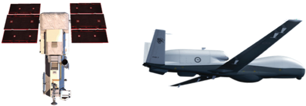
Figure 42: Left, a satellite (vector) with an on-board imaging radiometer (sensor) (source: DigitalGlobe); right, high altitude drone (vector) carrying a camera (sensor) (source: Aces Flying High).
